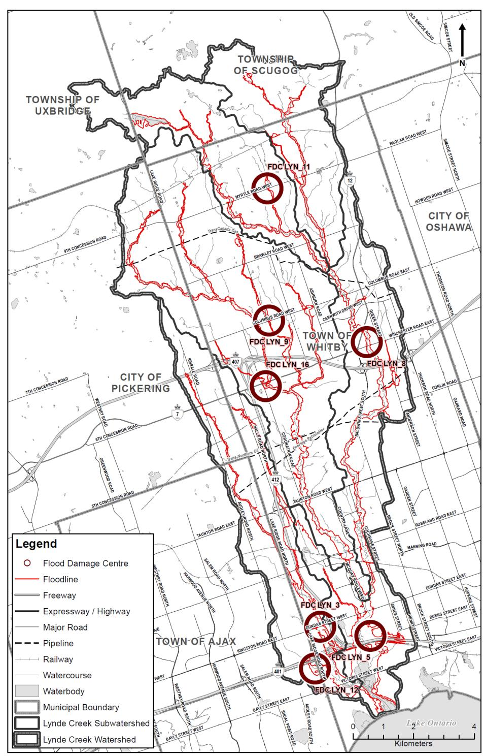
Figure 2-11: Existing Floodplain Mapping and Flood Vulnerable Areas
