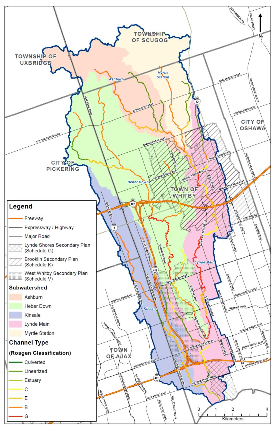
Figure 2-14: Identified Geomorphological Reaches within the Lynde Creek Watershed
